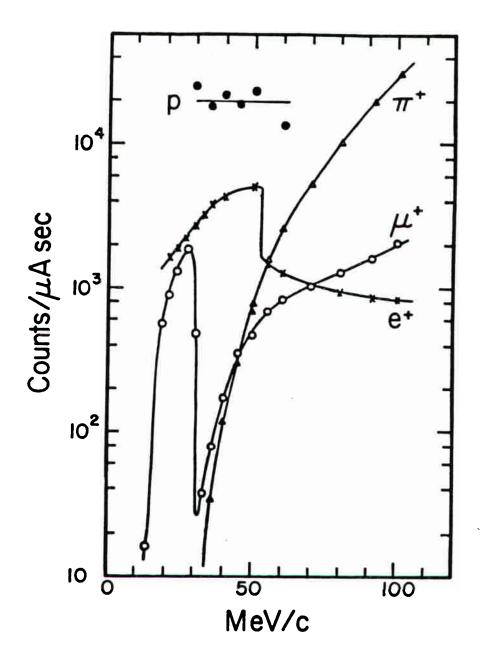
FIG. III.3. Positive particle fluxes versus beamline momentum settings in the M13 beamline at TRIUMF (taken from Ref. 26). The data was collected with all slits and jaws in the beamline fully open.
