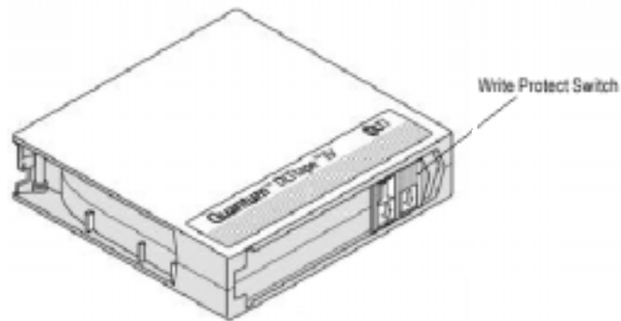
Figure B-5. Write-Protect Switch on Tape Cartridge
