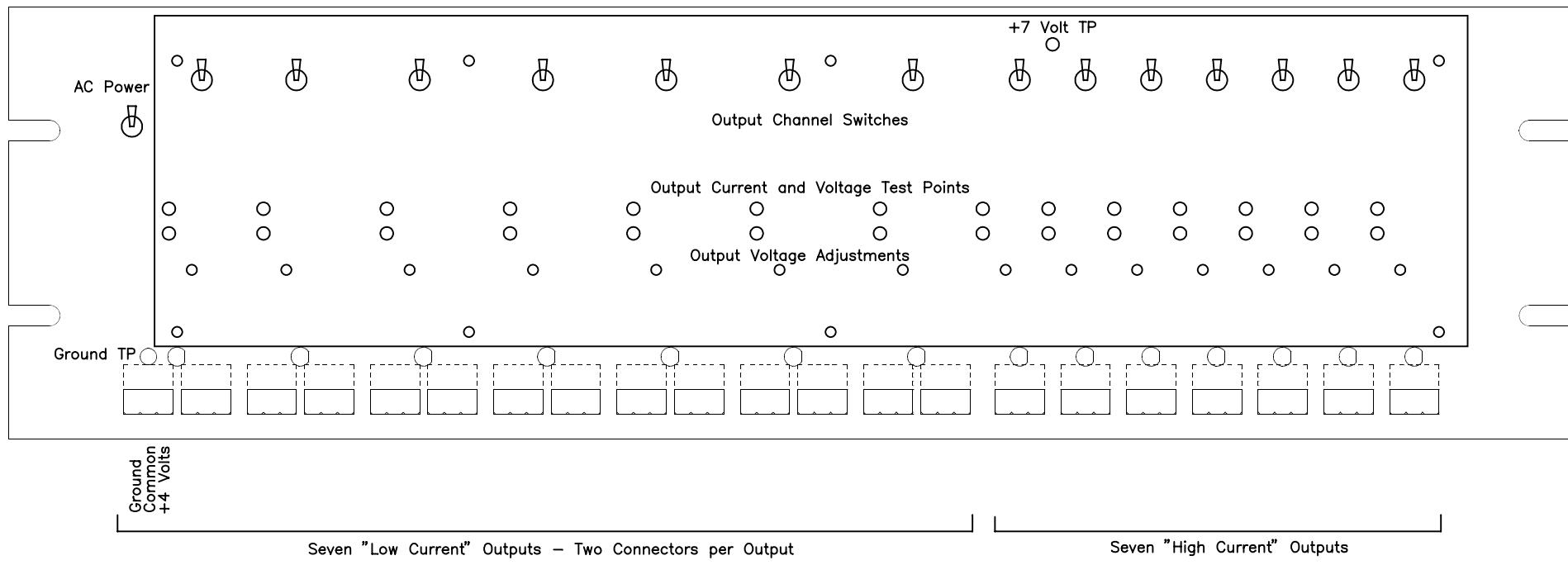
E614 Low Voltage Power Supply – Front Panel Layout
