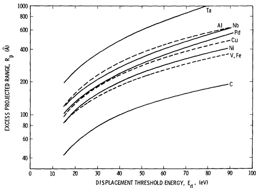
Fig. 1. Excess projected range as a function of displacement threshold energy for  $\mu^+$  projectiles incident on C (graphite), Al, V, Fe, Ni, Cu, Nb, Pd, and Ta.
