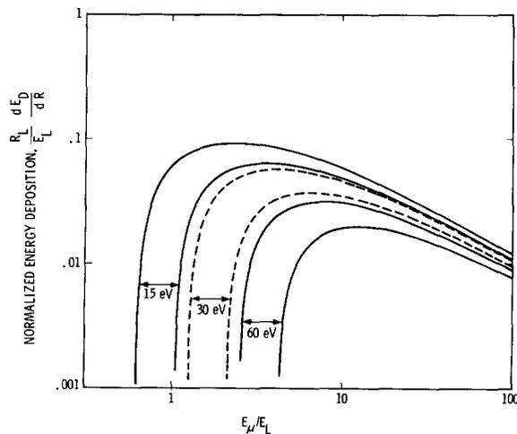
Fig. 2. Reduced rate of energy deposition into displacements for C and Ta targets as a function of reduced  $\mu^+$  energy for  $E_d = 15$  eV, 30 eV, and 60 eV. The upper curve in each set corresponds to the Ta target.
