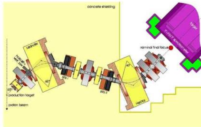
Figure 1.2: A schematic diagram of the *TWIST* beam-line
