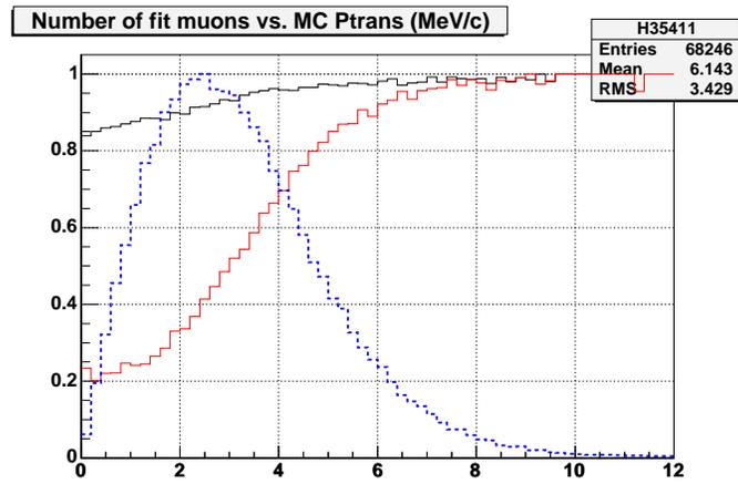
Figure 1.4: A comparison between the tracking efficiency vs. muon transverse momentum (MeV/c) before (red) and after (black) my changes to the pattern recognition software. The muon transverse momentum distribution is displayed in blue.
