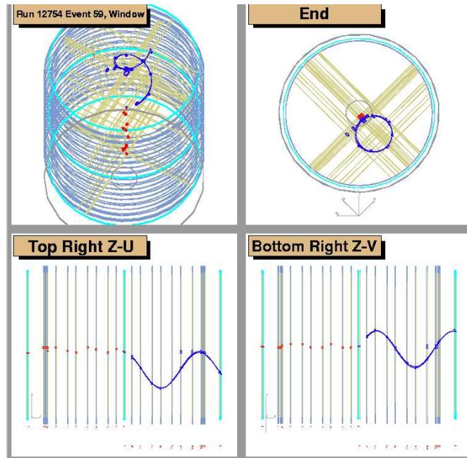
Figure 3.2: A visualisation of a typical negative muon decay event generated by the *TWIST* analysis software. The red tracks are the hits from the incoming muon. The decay electron hits are tracked to a helix, which is displayed in blue
