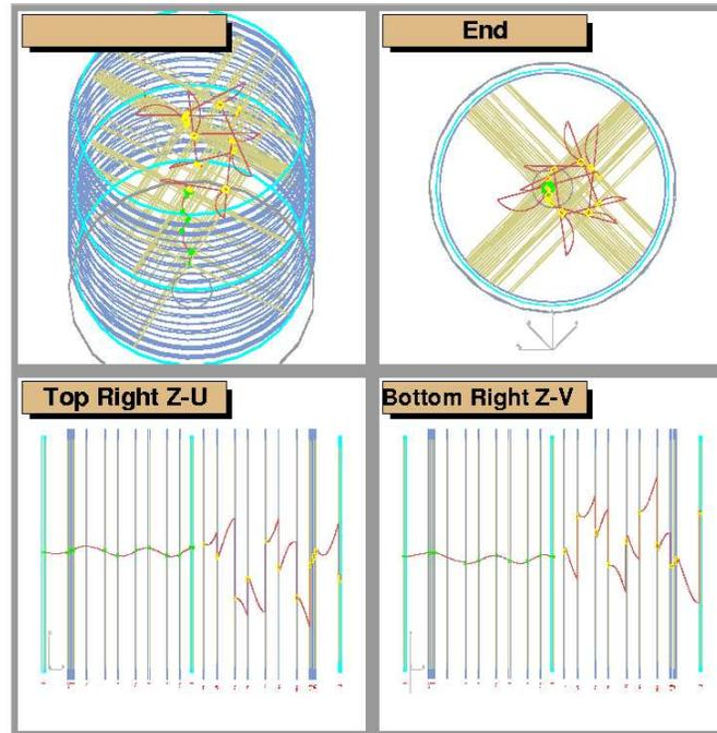
Figure 3.1: The above is a visualisation of a simulated  $\mu^+ \rightarrow e^-$  decay event in which the  $e^-$  was not tracked properly by the existing *TWIST* software. The failure of the analysis was obvious because the red analysis tracks are discontinuous at each of the DC planes
