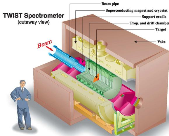
Figure 1.3: A schematic diagram of the *TWIST* spectrometer.
