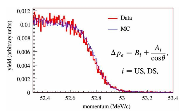
Spectrum endpoints for data and simulation differ by ~10 keV/c due to different stopping distributions, target thickness, magnetic field map scale.
