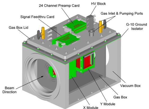
Figure 2: The TWIST TECs.
