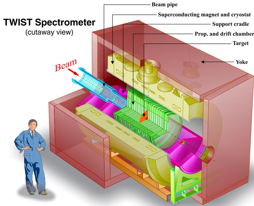
**FIGURE 1.** The TWIST spectrometer.
